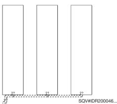
Composition example: 3 SQV#IDR200046 Total thermal yield: 3 x 717 Watts = 2151 Watts
