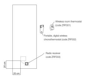
CONNECTION TO THERMOSTAT OR WI-FI\* CHRONOTHERMOSTAT (sold on request) Install a box that houses the "1" receiver which must be connected to the electric power supply and to the connection cable of the resistor. The receiver puts the Square electric version in contact with the thermostat and/or chronothermostat for radiator start up, adjustment and switch off.
