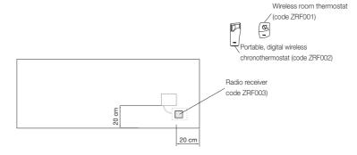
CONNECTION TO THERMOSTAT OR WI-FI\* CHRONOTHERMOSTAT (sold on request) Install a box that houses the "1" receiver which must be connected to the electric power supply and to the connection cable of the resistor. The receiver puts the Square electric version in contact with the thermostat and/or chronothermostat for radiator start up, adjustment and switch off.
