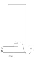
CONNECTION to electric SOCKET You must fit a plug (not supplied) to the pre-installed electric cord and arrange for an electric socket nearby. Even in this case we recommend a socket with switch
