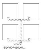
Composition example: 4 SQV#IDR060061 Total thermal yield: 4 x 361 Watts = 1444 Watts
