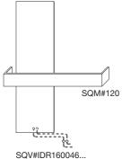
Composition example: SQV#IDR160046 + SQM#120 Total thermal yield: 596 Watts + 115 Watts = 711 Watts
